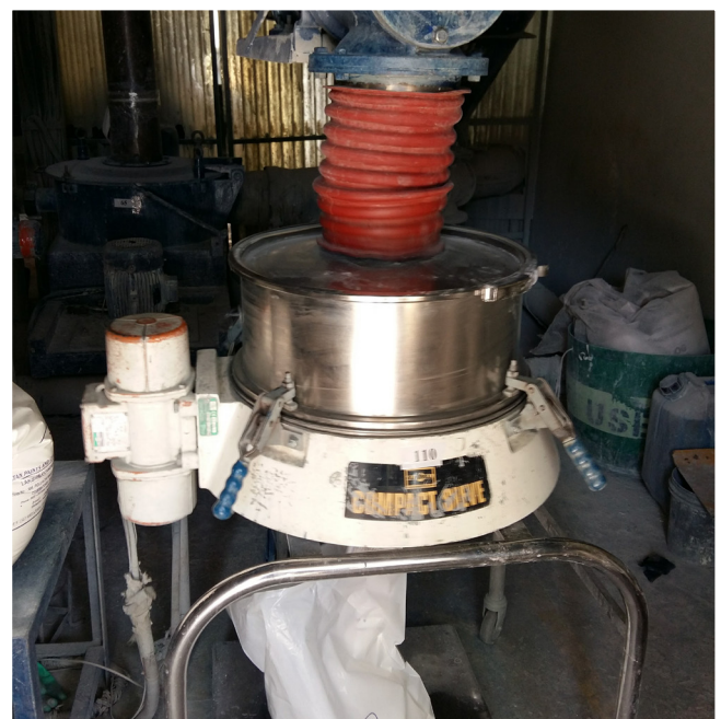
Figure 1. The Russell Compact Sieve® with Vibrasonic® Deblinding System is installed at the leading coatings company's plant
