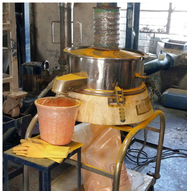
Figure 2. Sieving of powder coatings with the Russell Finex ultrasonic sieving solution at the company
