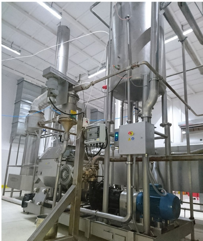
Figure 2. The Self-Cleaning Russell Eco Filter® with Russell Filter Management System™ provides an automated solution to filtering recovered frying oil.
