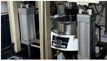
Installed in place of the metal detector, the Russell Compact Sieve® takes up less than 2 m² of floorspace. The vibratory action allows Realcafé to remove a wider variety of contaminants from the production process, including metallic and non-metallic materials; significantly improving the purity and quality of its product lines.
