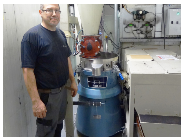
Picture 1. A Finex 22 Sieve™, installed at Fremach to optimize the flock reclaim process.
