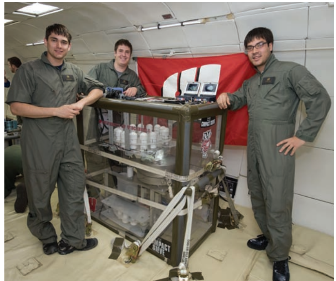
Figure 1. The test-rig containing the Russell Compact Sieve® to carry out the experiments
