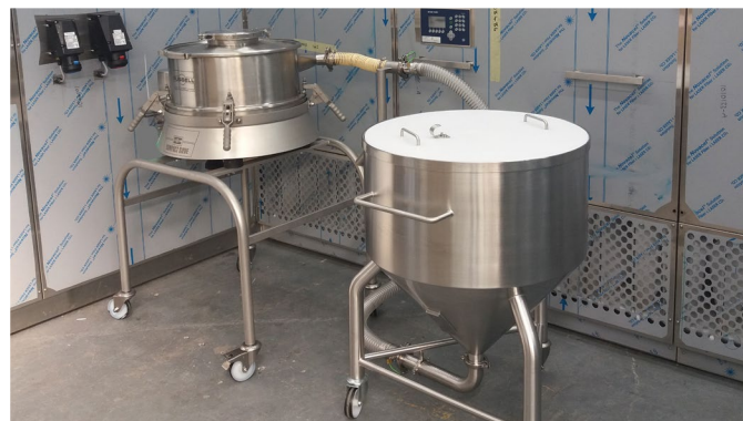
Figure 3. The Russell Compact Airswept Sieve™ installed in Howorth's WORKSAFE™ containment booth.
