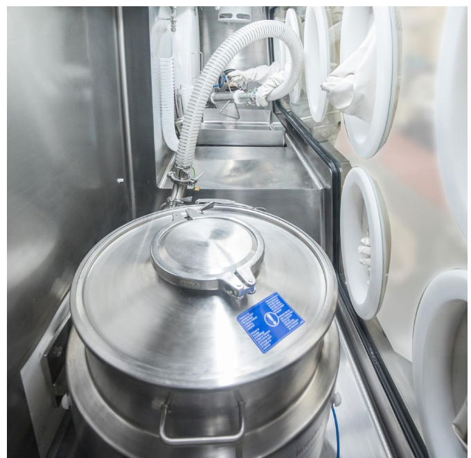
Figure 1. The Russell Compact Airswept Sieve™ fits easily inside a Containment Isolator.
