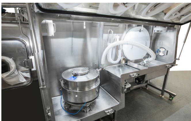
Figure 2. The Russell Compact Airswept Sieve™ with Russell Compact Airlock Sieve™ clamping system installed in a Howorth High Containment Isolator.
