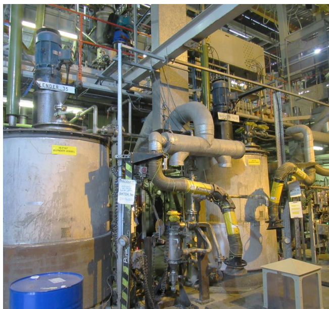
Figure 2. The Self-Cleaning Russell Eco Filter® at Lucite is used to remove agglomerates from an adhesive resin used for surgical plasters
