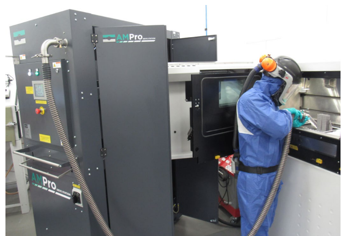
Figure 1. The Russell AMPro Sieve Station™ is used to reclaim and requalify AM powders from the build process at Progressive Technology.
