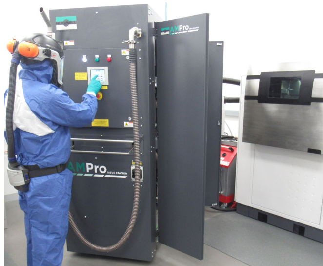
Figure 2. The key to the Russell AMPro Sieve Station™ is how every detail has been designed and incorporated into a fully-automated one-button process.
