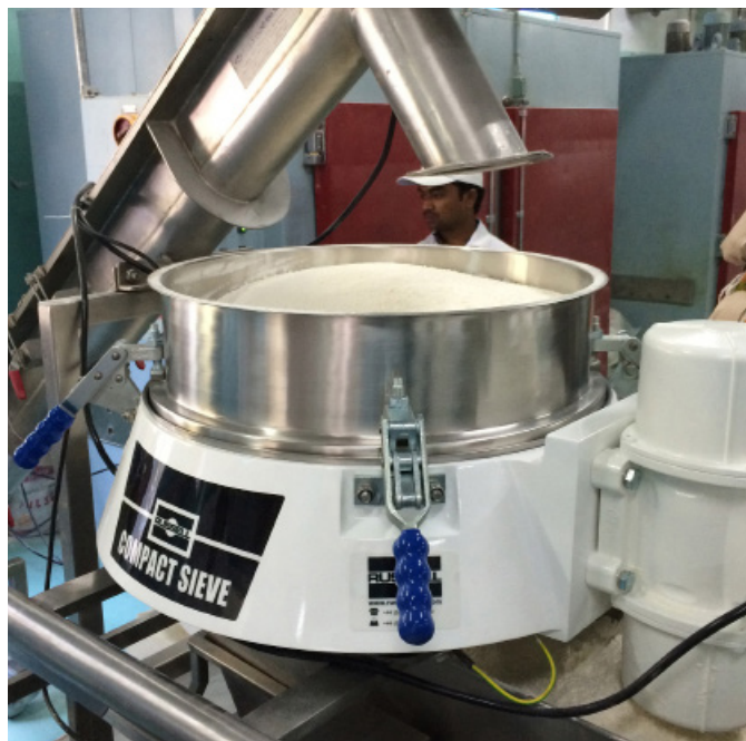
Figure 2. The Russell Compact Sieve® installed as a final quality check before packaging
