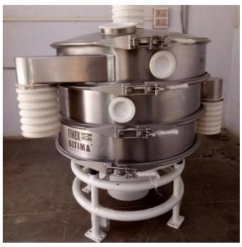
**Figure 2.** The Finex Ultima<sup>™</sup> has a high-clean open frame design.
