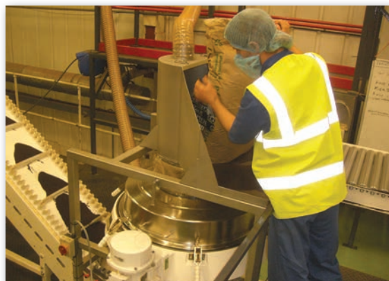
Figure 3. The Compact 3in1 Sieve™ bag tipping station used to load 75 kilo bags of tea
